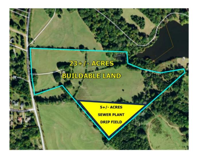
Based on 200 Units, we estimate that this project will use our 50,000 gallon a day High-Tech "STEP" Sewer System. The materials (Tanks and Drip Field) would only cost about \$3,000.00 per Unit.
